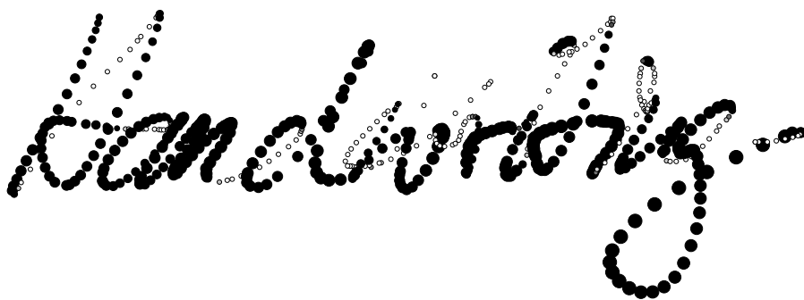
Fig. 2.6. Example of a pen trajectory of the handwritten word “ handwriting ” captured online. The size of the dots representing the pen positions encodes the pen pressure in pen-down strokes (black) and the shading represents the distance to the writing surface during pen-up movements.
